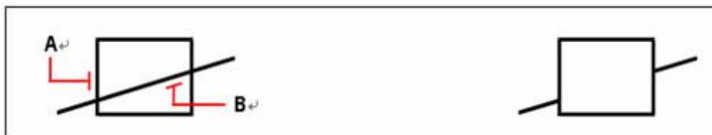
To trim objects, select the cutting edge (A), and then select the objects to trim (B)
